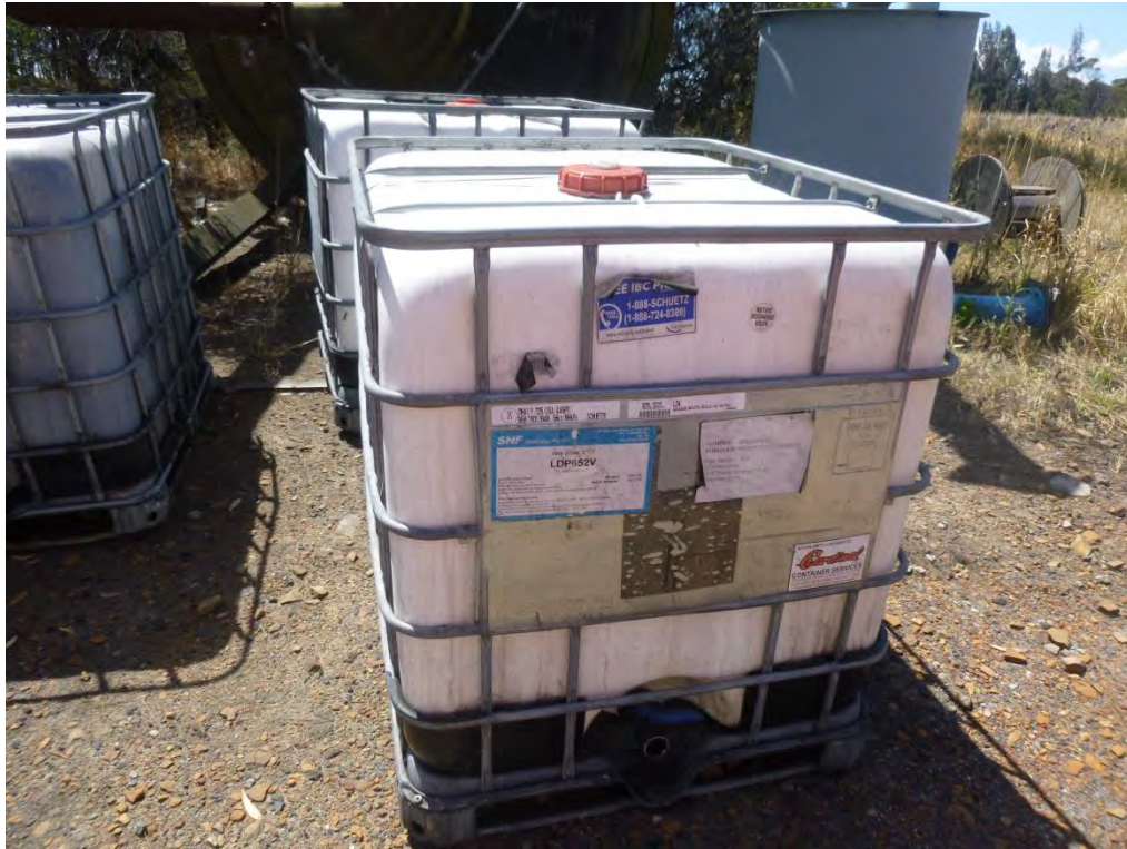
Photo 1 – Self bunded chemical containers
