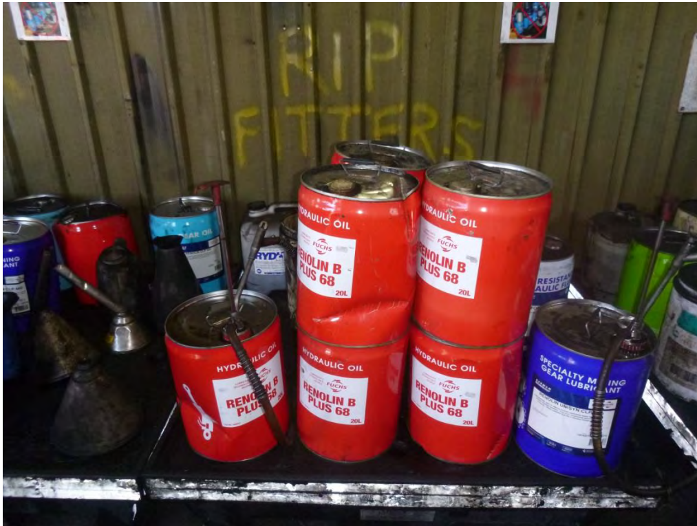
Photo 7 – Drums should not be stacked
