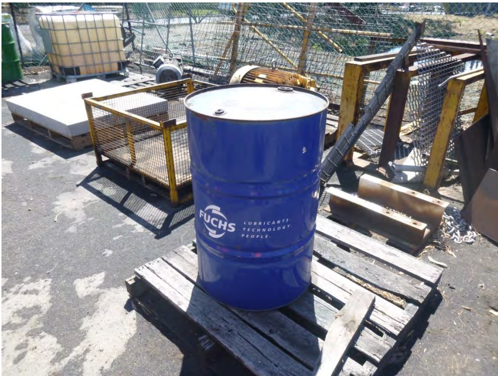
Photo 6 – Unbanded drum near workshop
