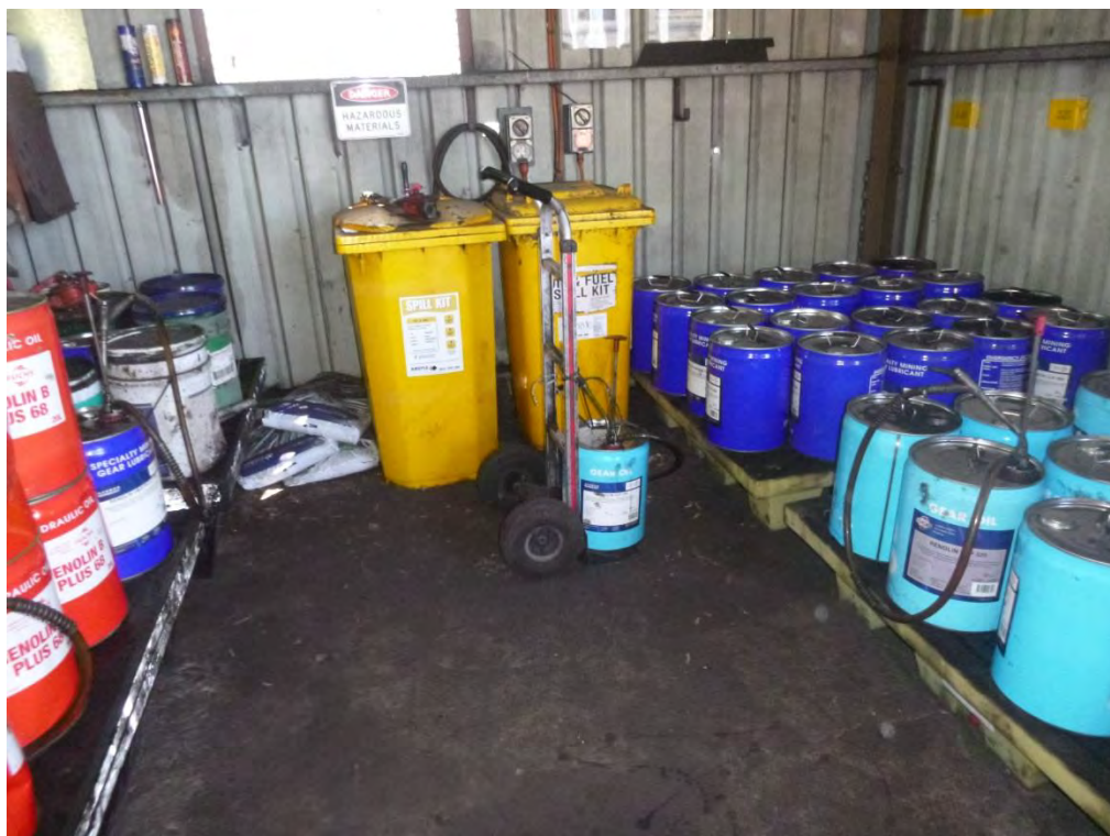
Photo 8 – Spill kit and banded drums.
