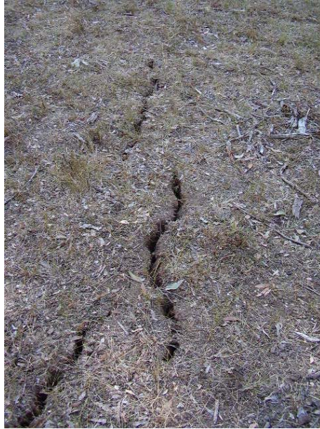
Fig. 4.10 Surface Tension Cracking along the Top of a Steep Slope
