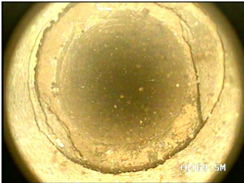
Appendix 6.6: 169.3m - Water loss zone, near horizontally orientated joint zone.
