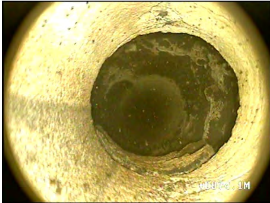
Appendix 6.1: 74.8m - Core loss zone, Large cavity present in the Hawkesbury Sandstone.
