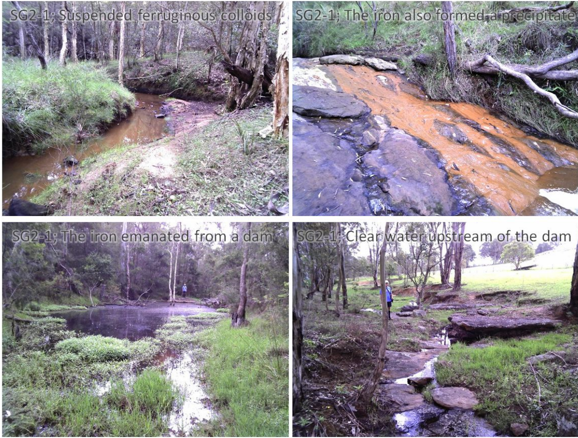
Figure 53. Ferruginous colloids suspended in the water of Sugarloaf Gully over a 310 m long reach. Photographed 13 February 2013.
