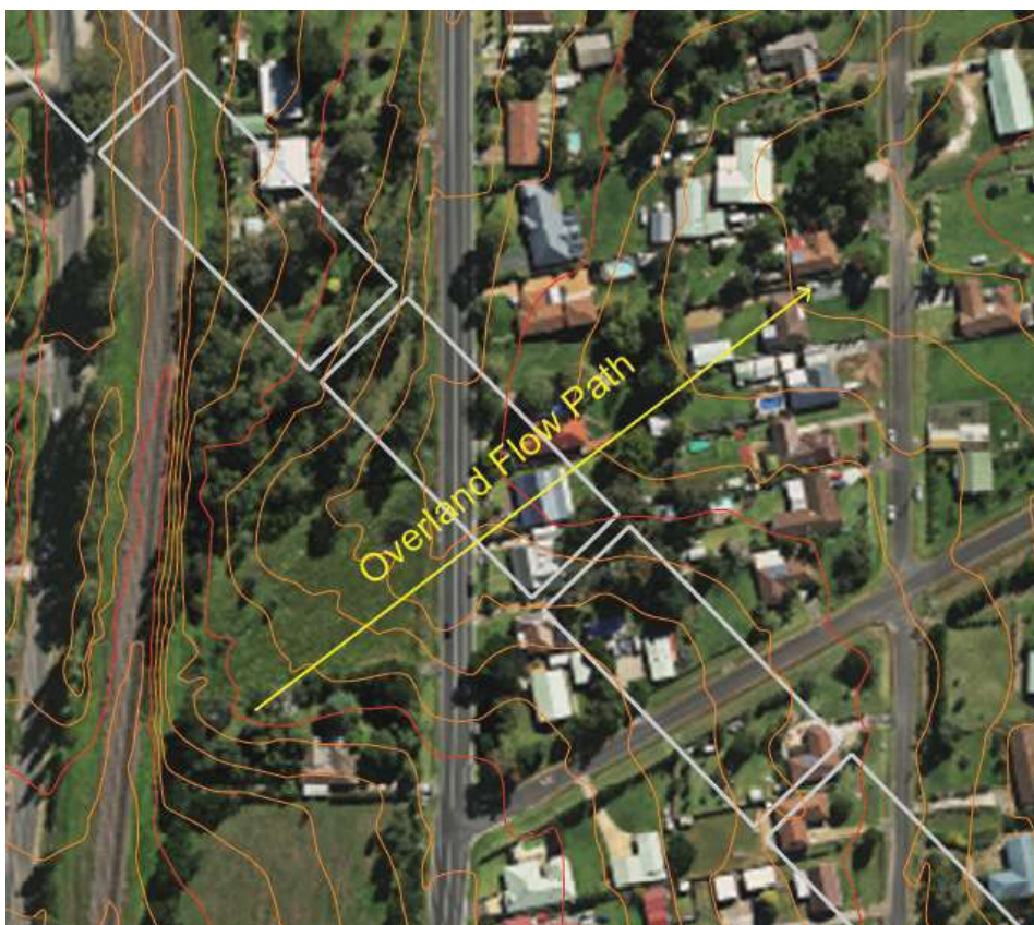
Figure 20 Overland Flow Path Between Railway and Great Southern Road
