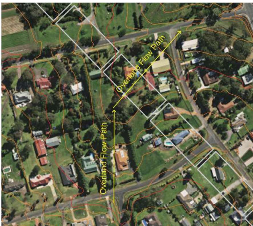
Figure 18 Overland Flow Path South of Wellers Road
