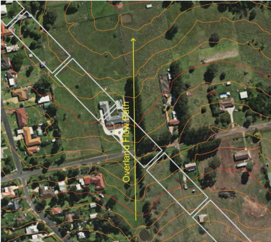
Figure 17 Overland Flow Path North of Bargo Road
