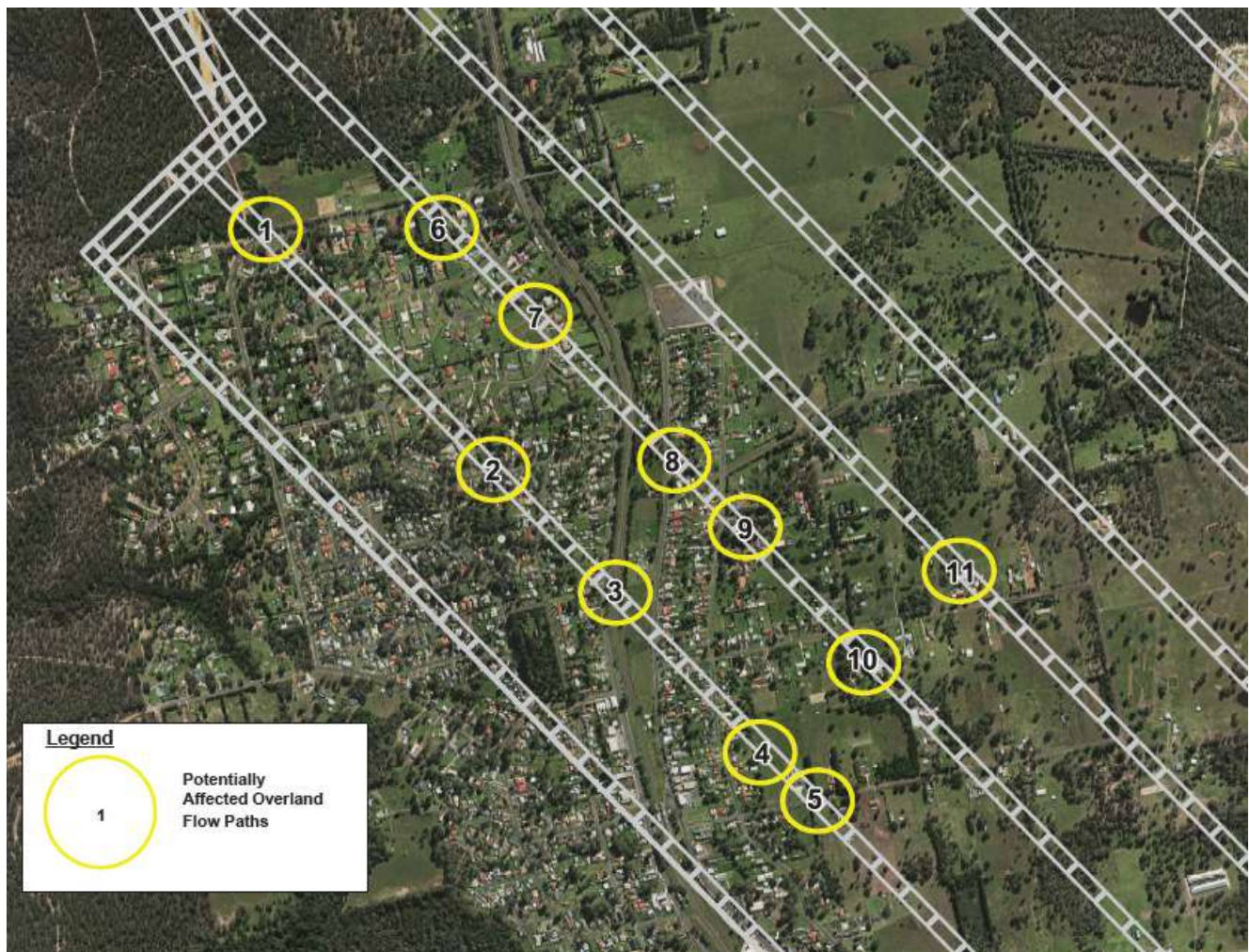
Figure 12 Proposed Longwall Panel Layout – Bargo Township and Potentially Affected Overland Flow Paths
