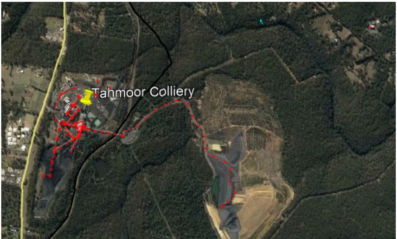
Figure B.1 Indicative noise source locations for noise modelling – Existing Tahmoor mine
