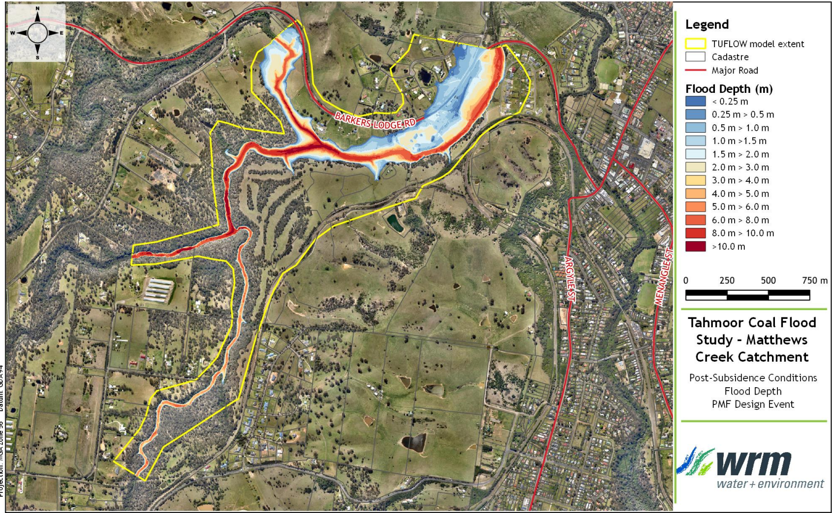
Figure B.3 - Matthews Creek catchment post-subsidence conditions - PMF event flood depth
