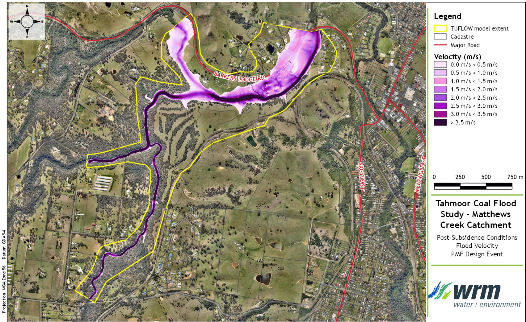
Figure B.4 - Matthews Creek catchment post-subsidence conditions - PMF event velocity
