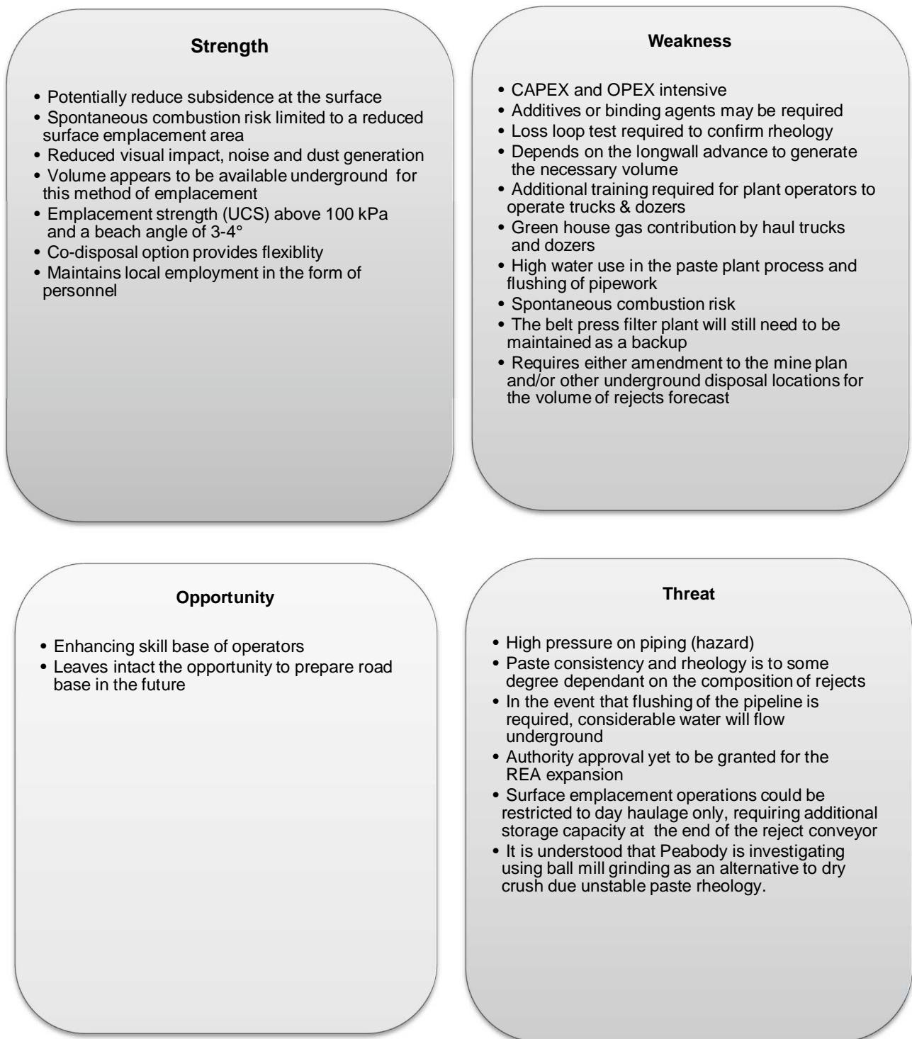
Figure 7-12 SWOT analysis, Co-disposal Option – REA Expansion plus UG disposal – paste material (active goaf via trailing pipe)
