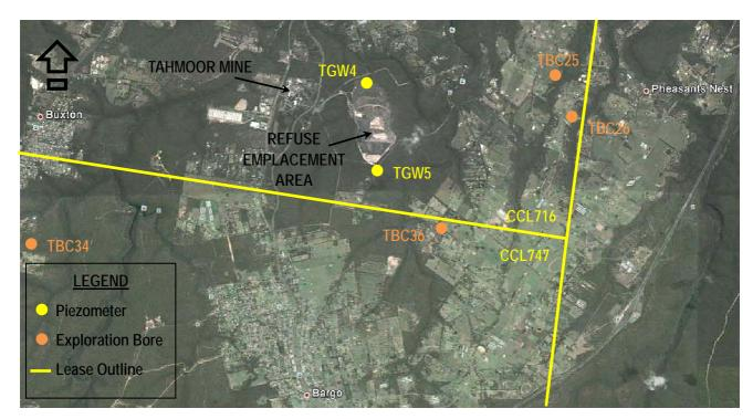
Figure 2 Exploration and Piezometer Bore Locations
