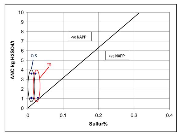
Figure 5 Total Sulfur and Sulfide Sulfur Acid Base Account
