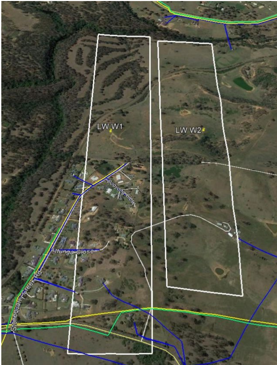
Plate 1: Google Earth aerial view of two longwalls LW W1-W2 showing Thirlmere Way in the south and Barkers Lodge Road in the north. The green lines indicate NBNCo optical fibre cables, south between Picton and Tahmoor exchanges and along Stonequarry Creek Road and north along Barkers Lodge Road between from Picton and west. The blue lines are the NBNCo local copper customer cables and the yellow lines are the Telstra IEN optical fibre cables.
