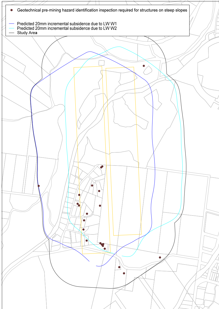
Fig. 5.2 Locations of structures on or near steep slopes
