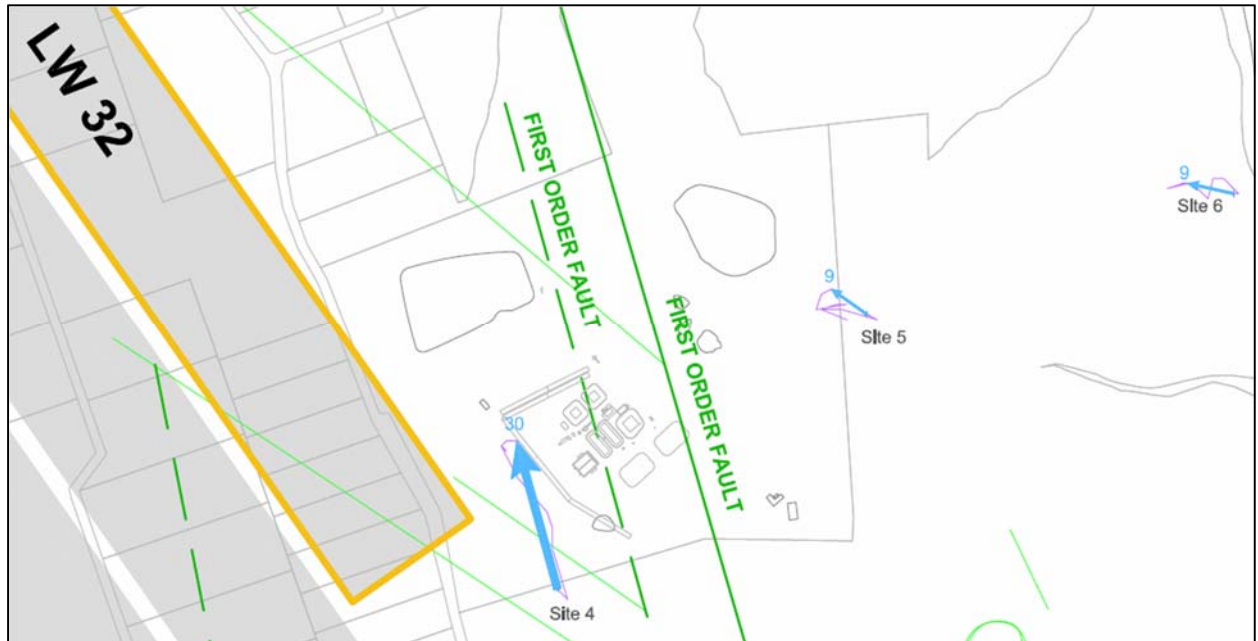
Fig. 2.16 Observed horizontal movements at the PWRP GNSS units during the mining of LW 32
