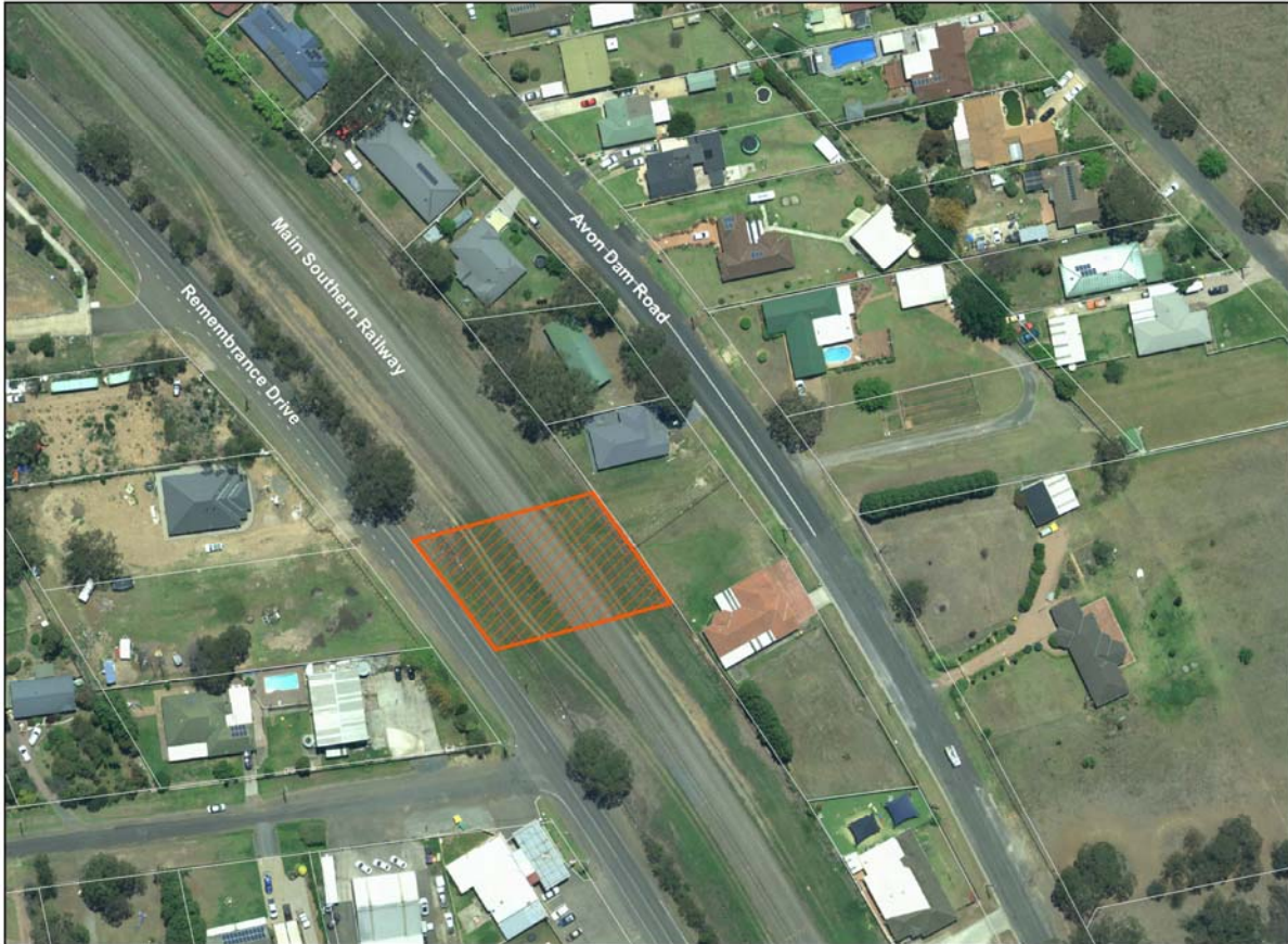
Fig. 6.21 Aerial photo, marked to show the position of buried gas and ethane pipelines beneath Remembrance Drive and Main Southern Railway (LW106B ~660m to north east)
