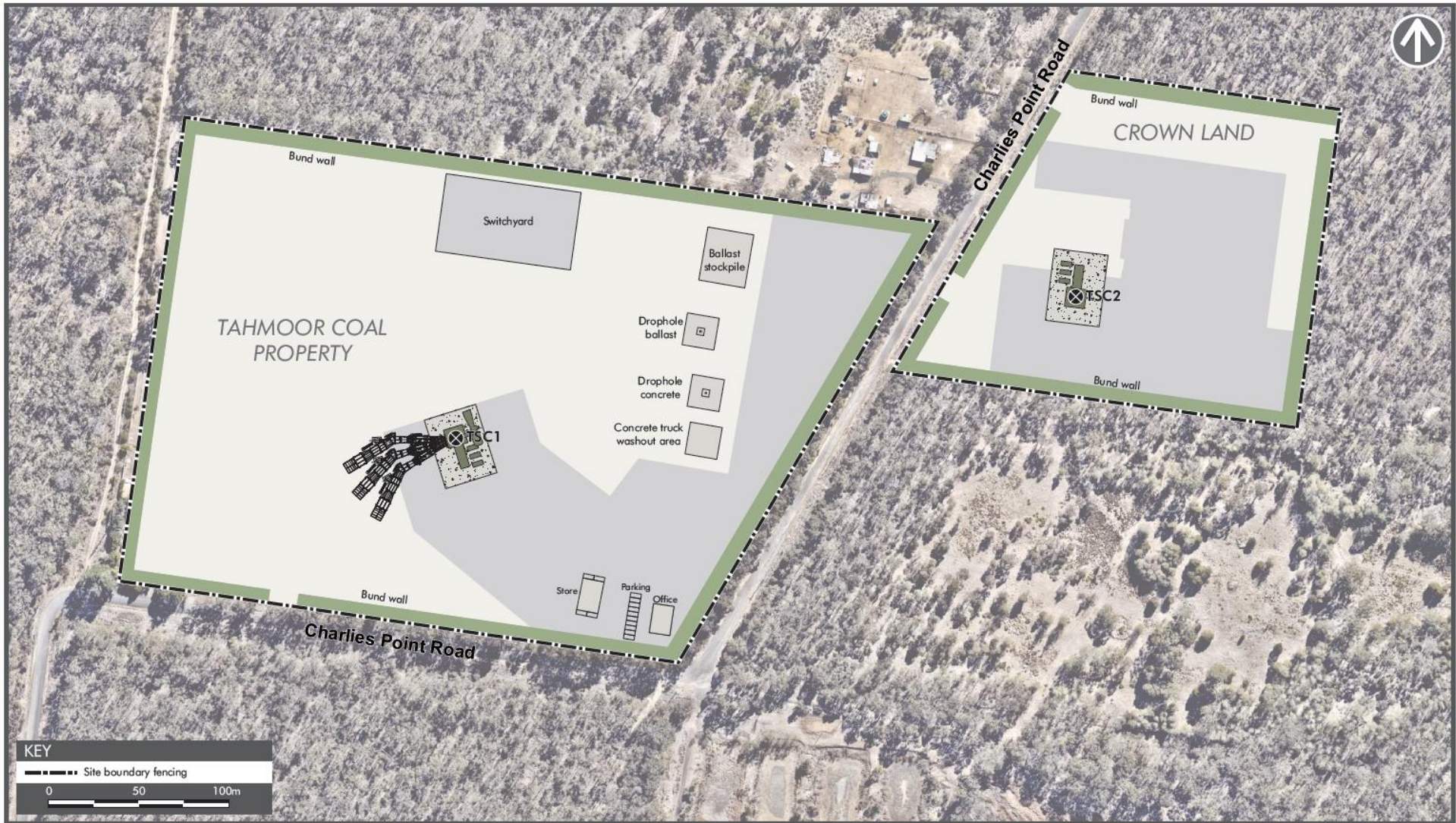
Figure 13 Proposed Project Conceptual Ventilation Shaft Layout
