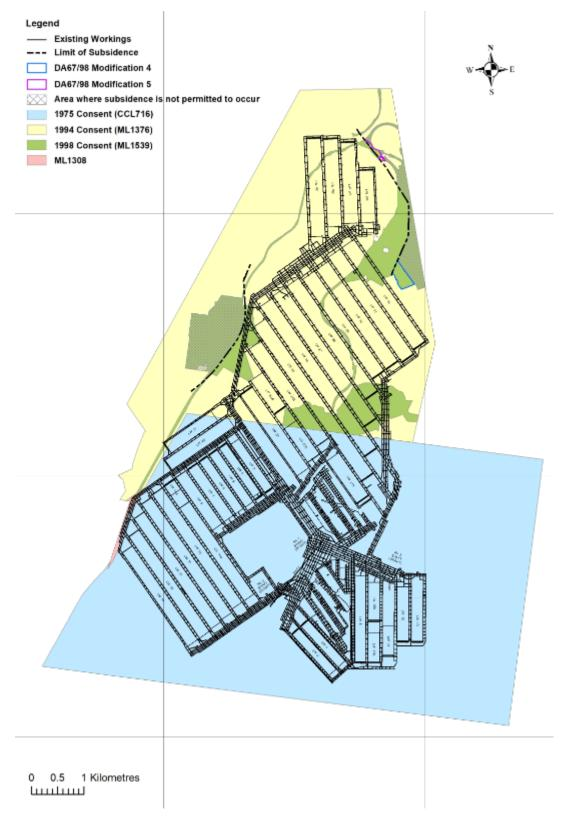
**Figure 2:** Map of Tahmoor Mine showing two areas (in black crosshatching) where subsidence is not permitted under condition 6(i) of this consent.
