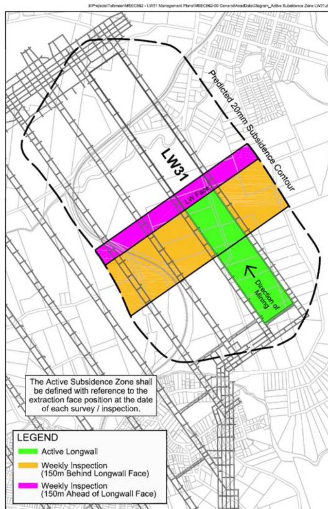
Fig. 1.1 Diagrammatic representation of the active subsidence zone
