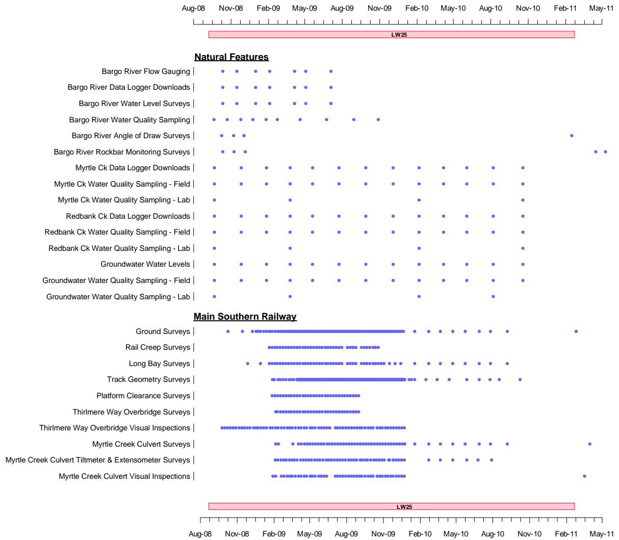
Fig. 3.2 Timeline of Surveys and Inspections during Longwall 25
