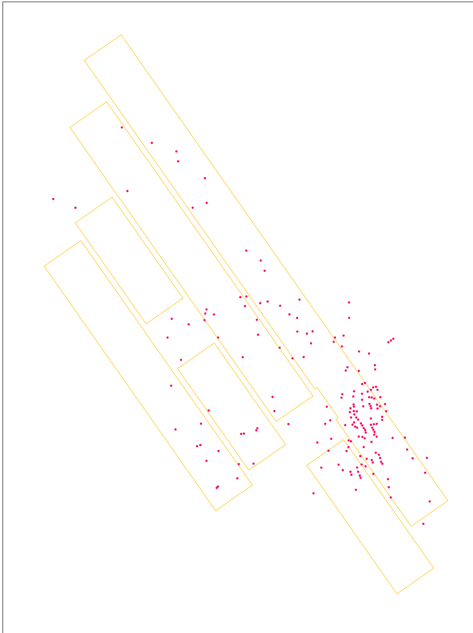
Fig. 4.4 Locations of Impacts Reported during the Mining of Longwall 25
