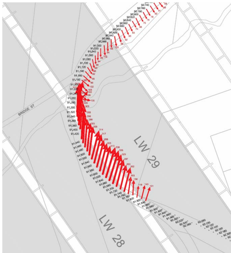
Fig. 2.8 Observed total horizontal movement along Main Southern Railway during the mining of Longwalls 27 to 29 as at 24 May 2016
