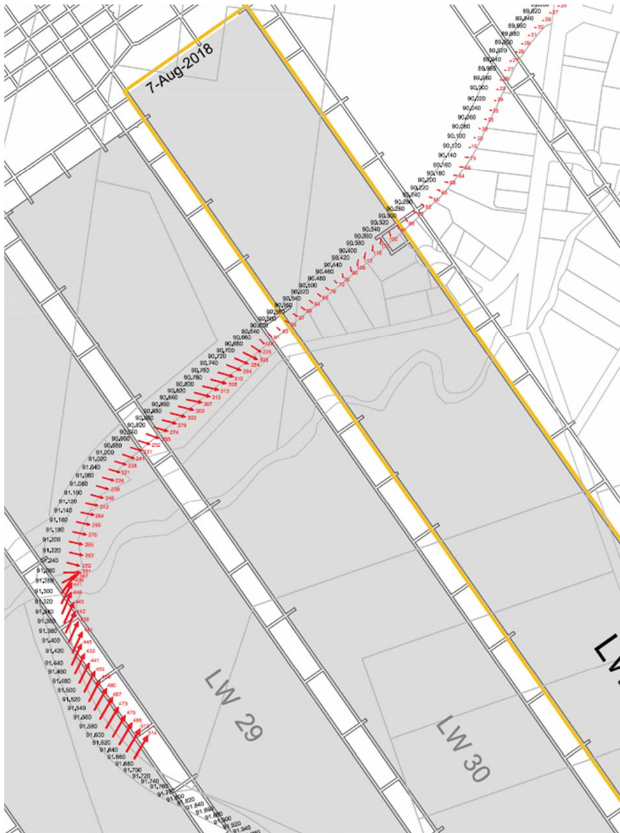
Fig. 2.7 Observed total horizontal movement along Main Southern Railway during the mining of Longwalls 27 to 31
