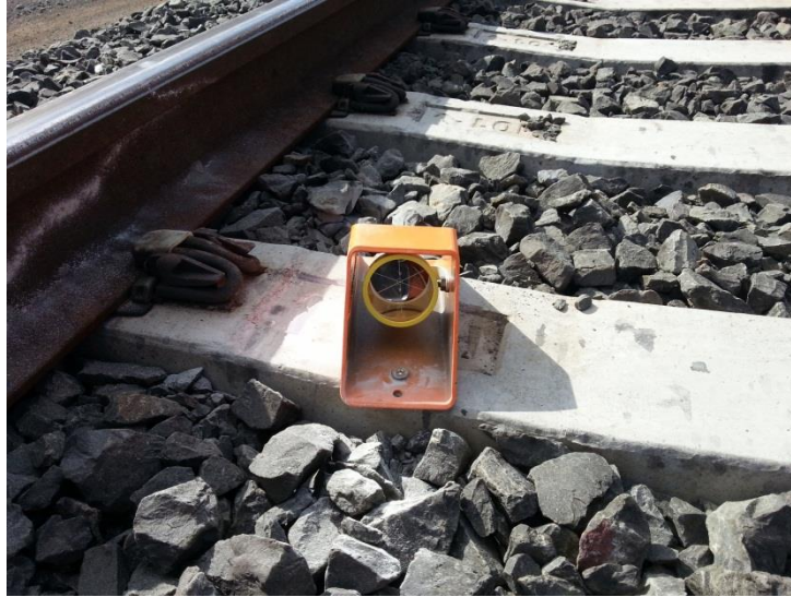
Fig. 2.6 Typical survey prism on railway sleeper
