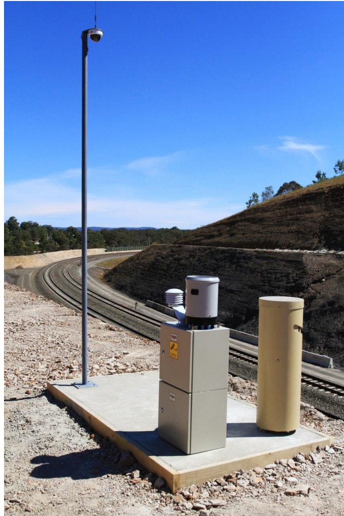
Fig. 2.4 Total Station 1 with weather station
