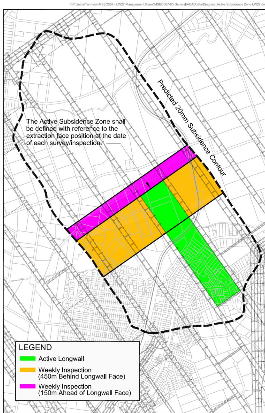
Figure 1.2 Diagrammatic Representation of Active Subsidence Zone
