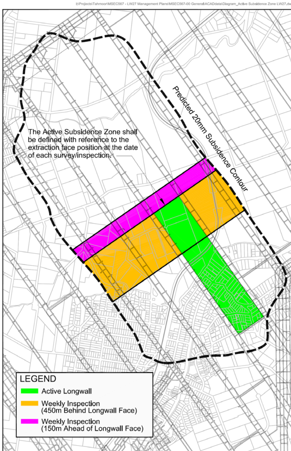
Fig. 1.1 Diagrammatic Representation of Active Subsidence Zone
