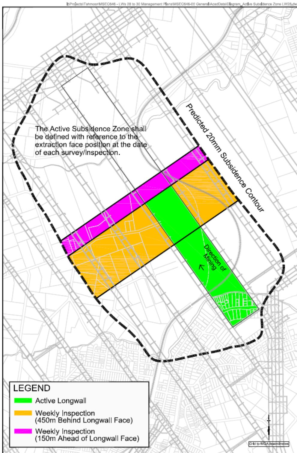
Fig. 1.1 Diagrammatic Representation of Active Subsidence Zone
