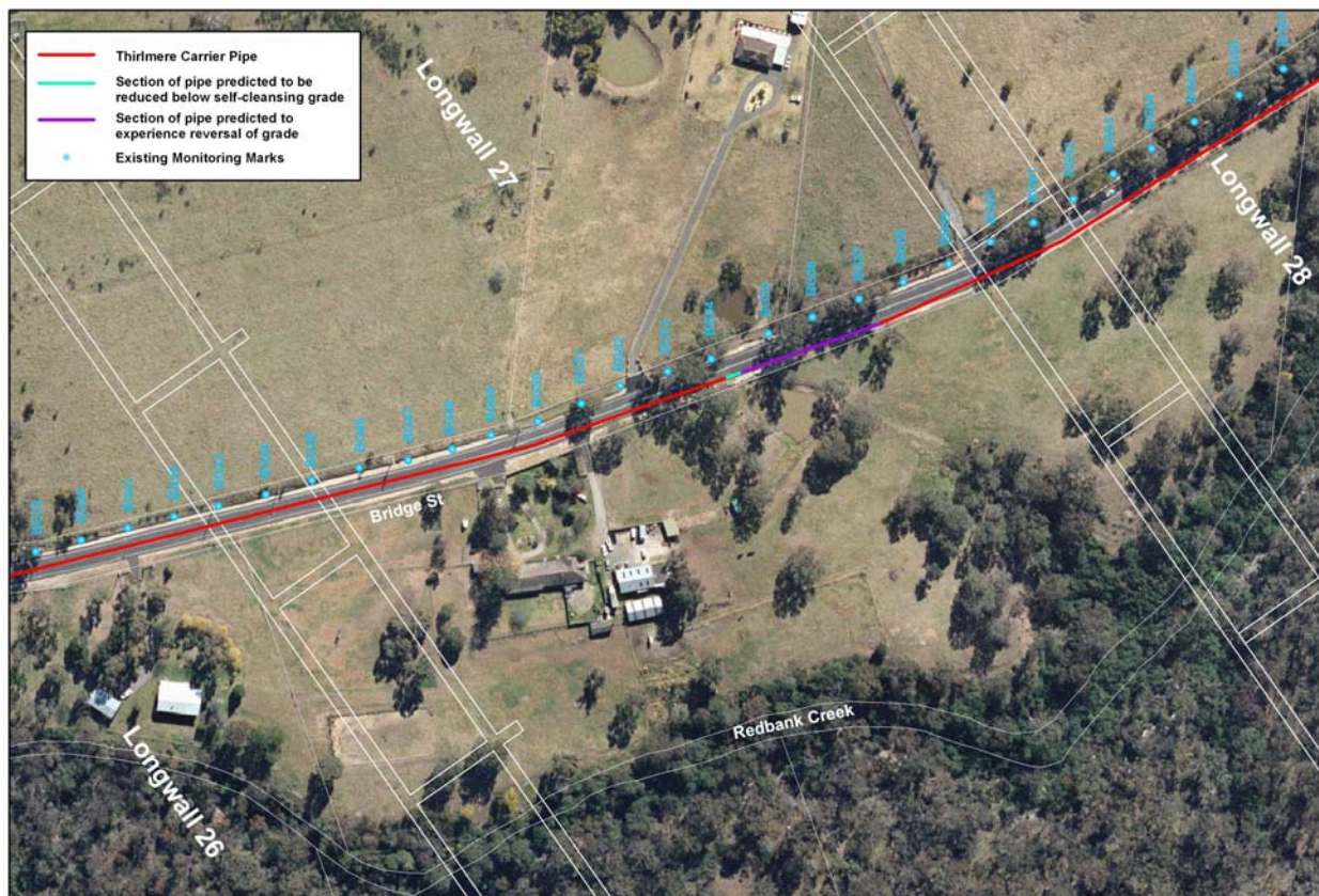
Fig. 2.16 Location of Thirlmere Carrier Pipe on Bridge Street where a reversal of grade may occur during the mining of Longwall 27
