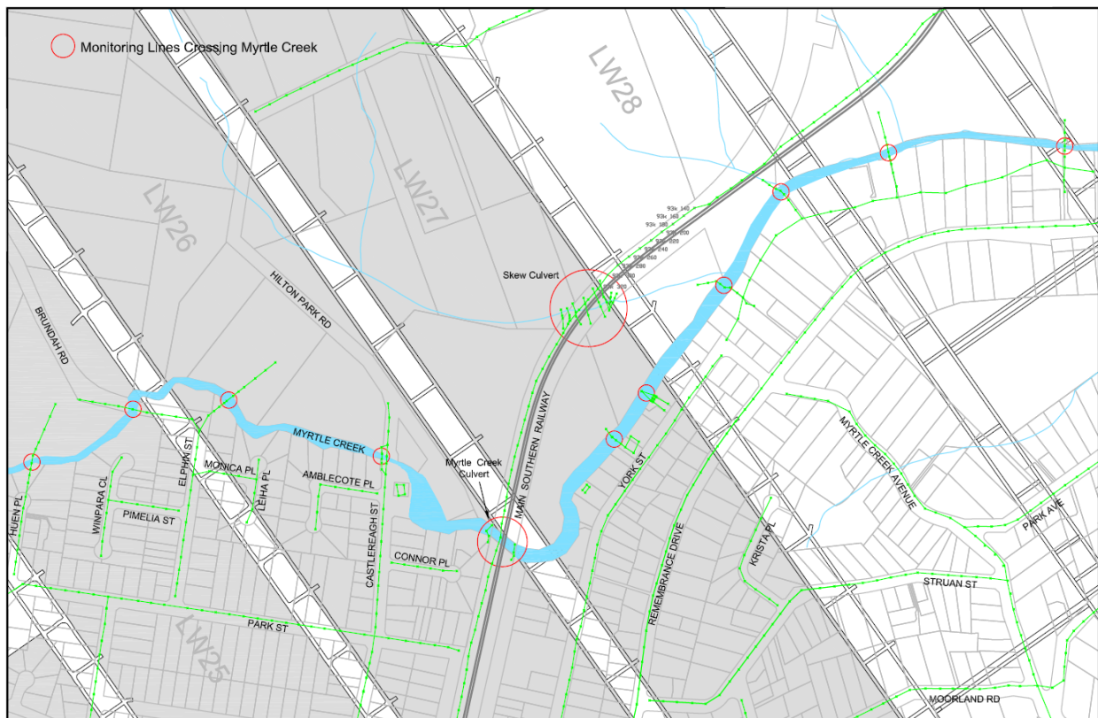
Fig. 2.8 Monitoring lines across Myrtle Creek and Skew Culvert
