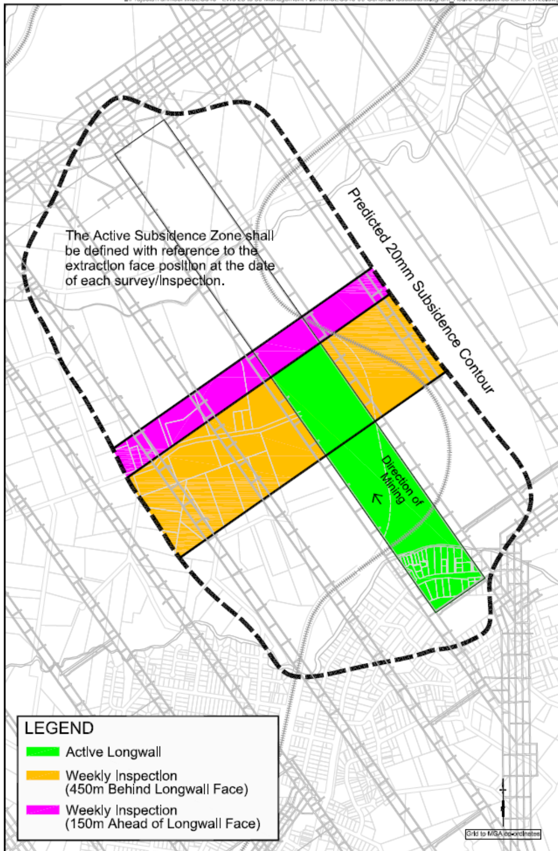
Fig. 1.1 Diagrammatic Representation of Active Subsidence Zone
