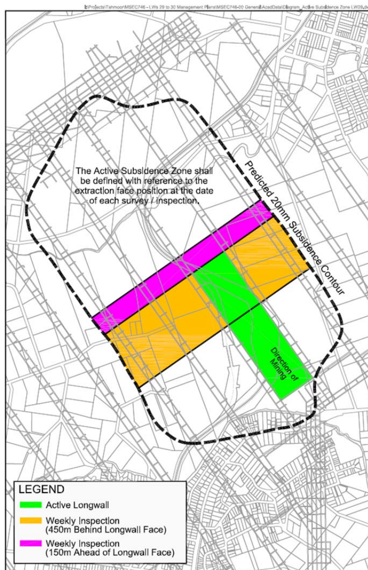
Fig. 1.1 Diagrammatic Representation of Active Subsidence Zone
