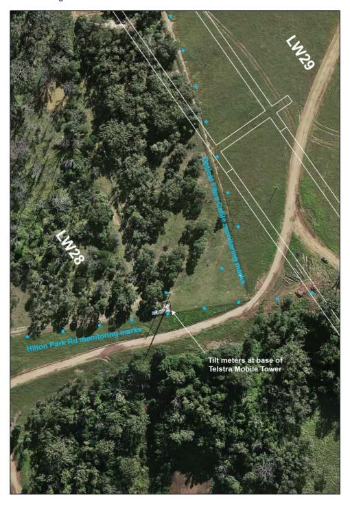
Fig. 2.13 Location of monitoring marks in vicinity of Telstra Mobile Tower
