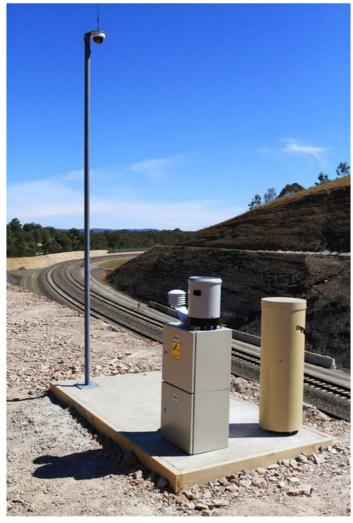
Fig. 2.3 Total Station 1 with weather station
