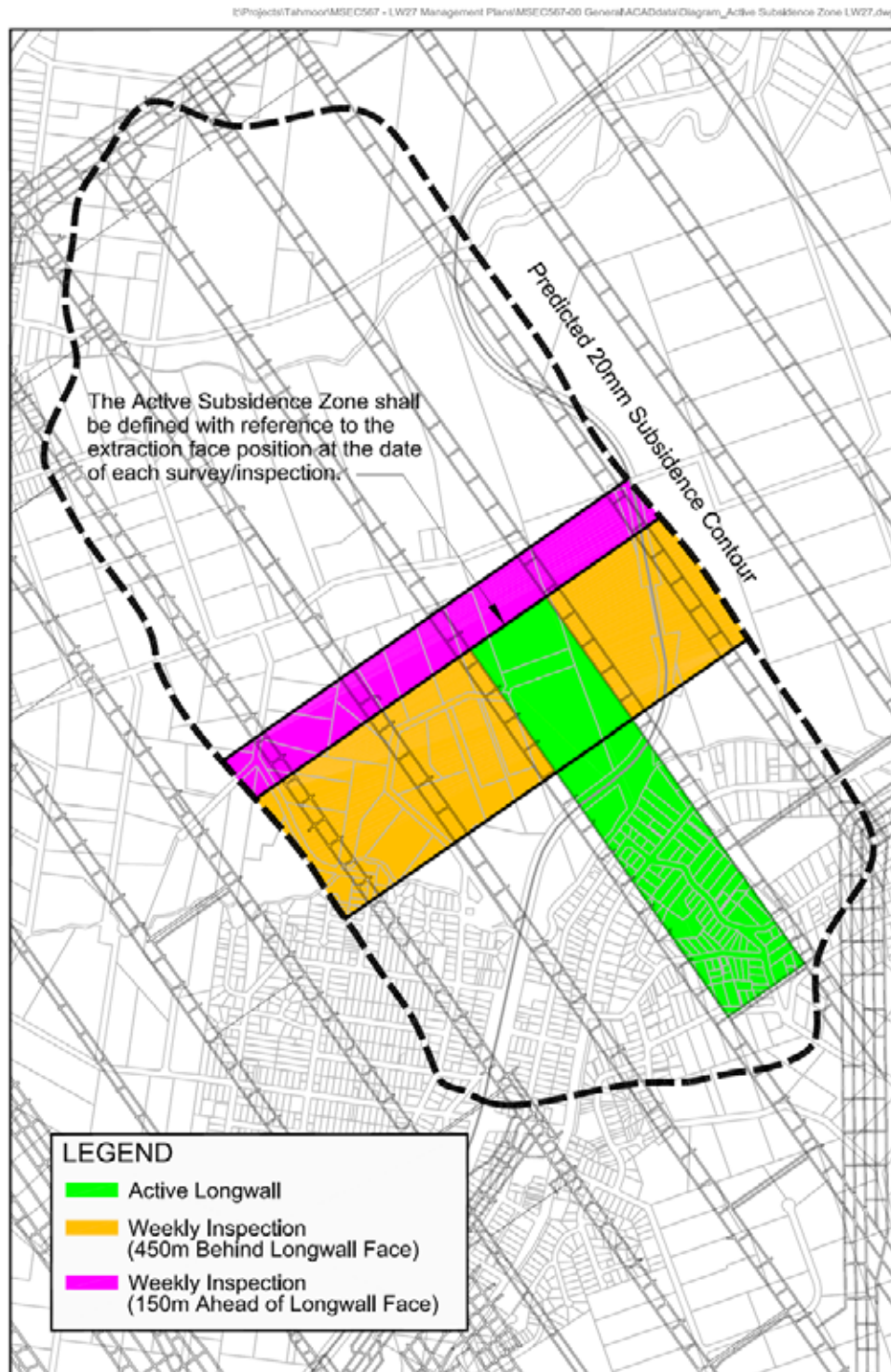
Fig. 1.1 Diagrammatic Representation of Active Subsidence Zone
