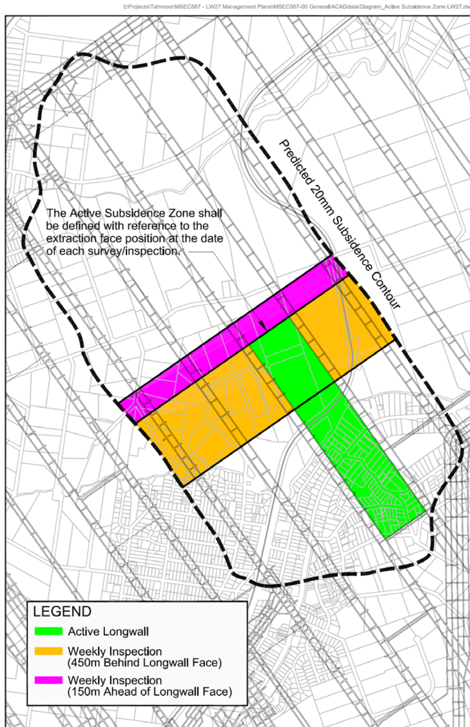
Fig. 1.6 Diagrammatic Representation of Active Subsidence Zone
