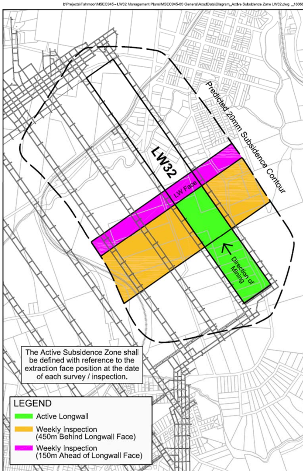
Fig. 1.2 Diagrammatic representation of the active subsidence zone
