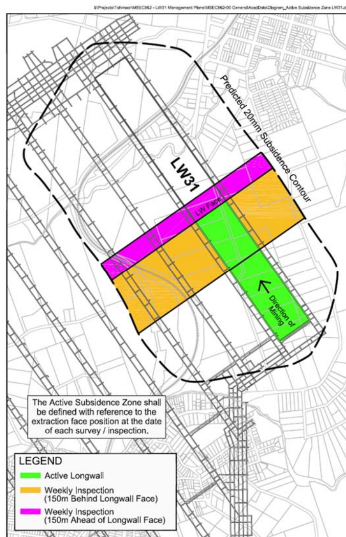
Fig. 1.1 Diagrammatic representation of the active subsidence zone
