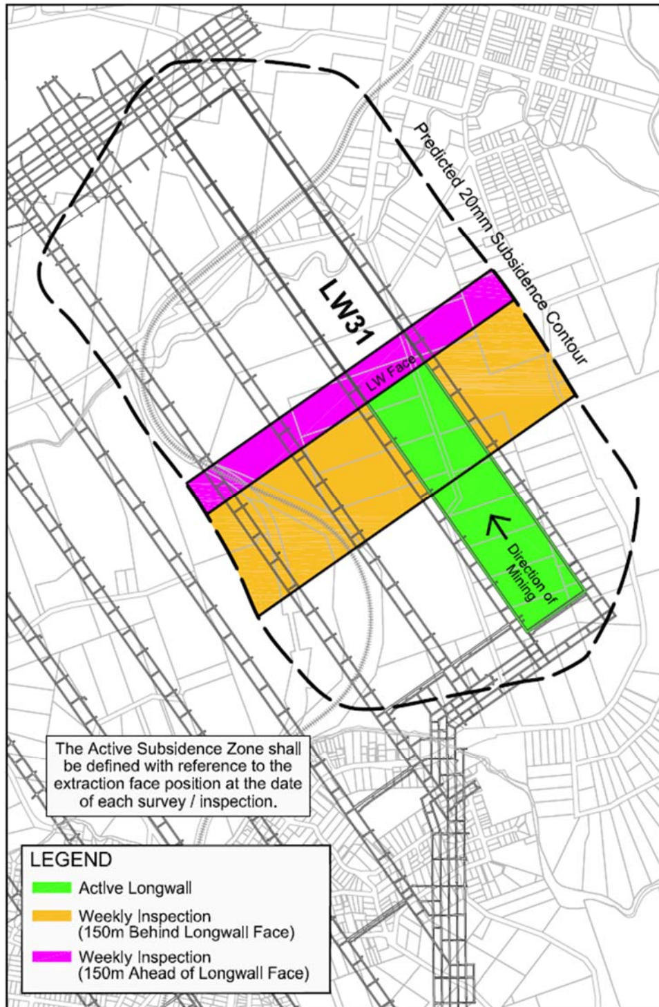
Fig. 1.1 Diagrammatic representation of the active subsidence zone
