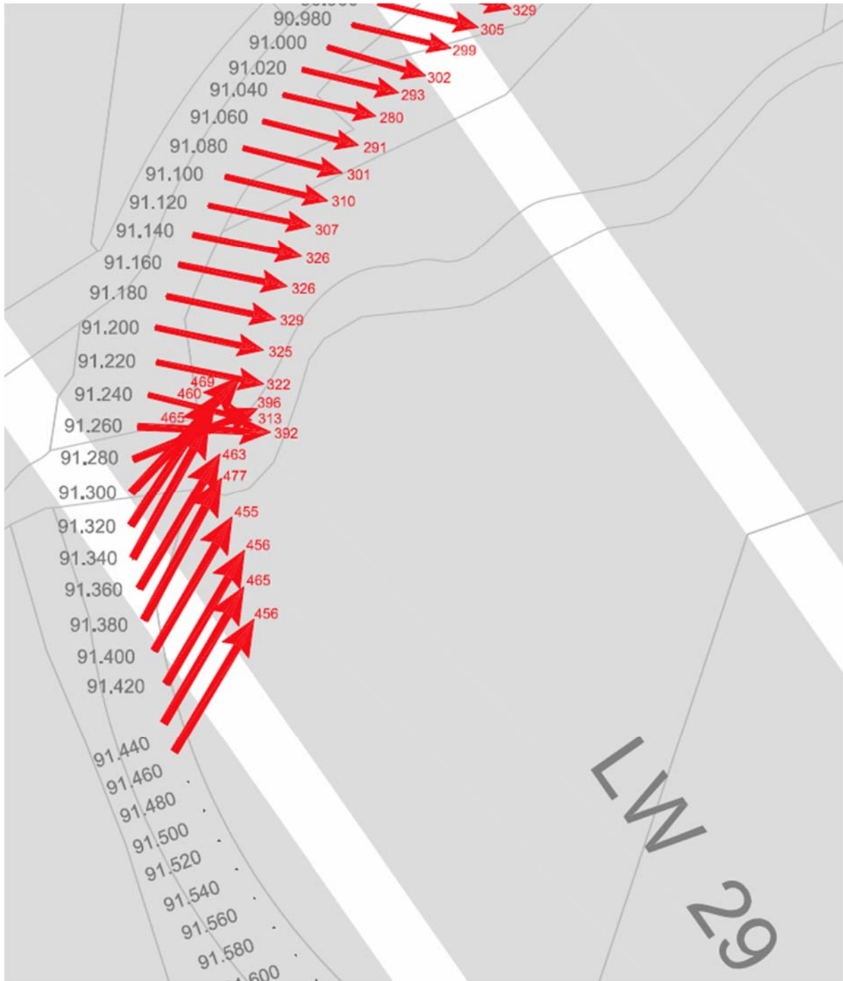
Fig. 2.6 Observed total horizontal movement along Main Southern Railway during the mining of Longwalls 27 to 32
