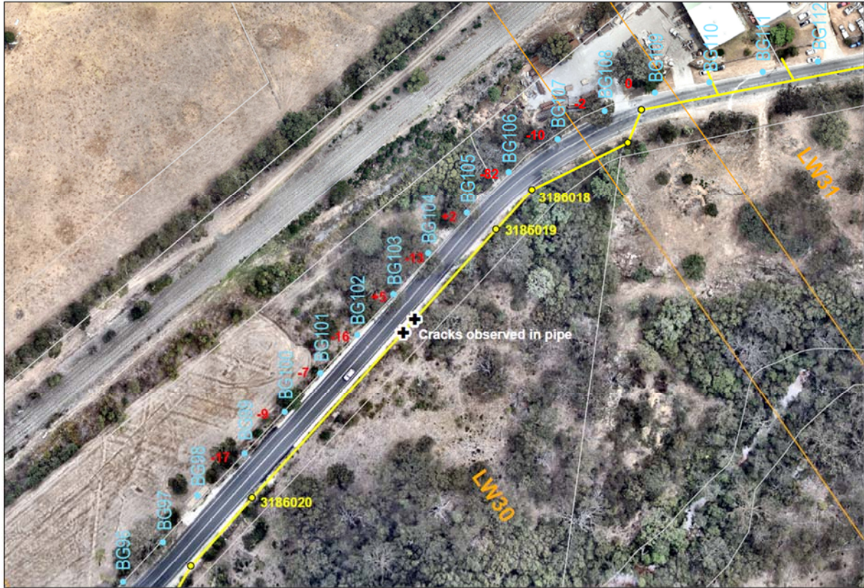
Fig. 4.4 Locations of cracks observed by CCTV inspection in Thirlmere Carrier Pipe on 25 July 2018
