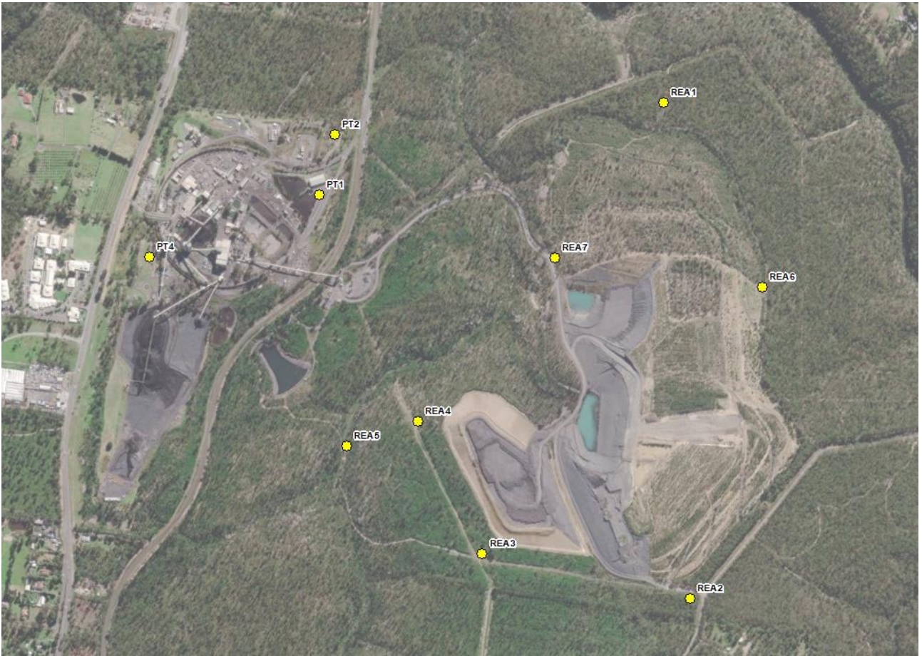
Figure 11 Locations of Piezometers at Pit top and the REA
