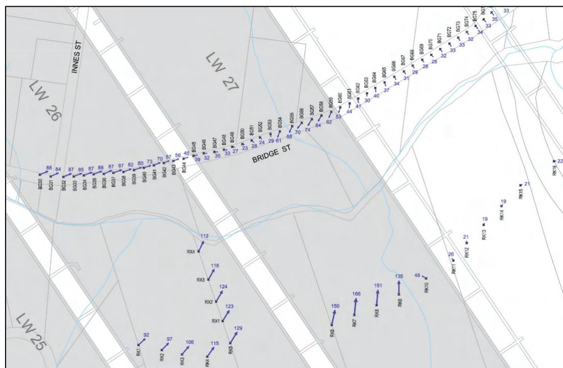
Fig. 3.19 Observed Relative Horizontal Movements across Redbank Creek during Longwall 27
