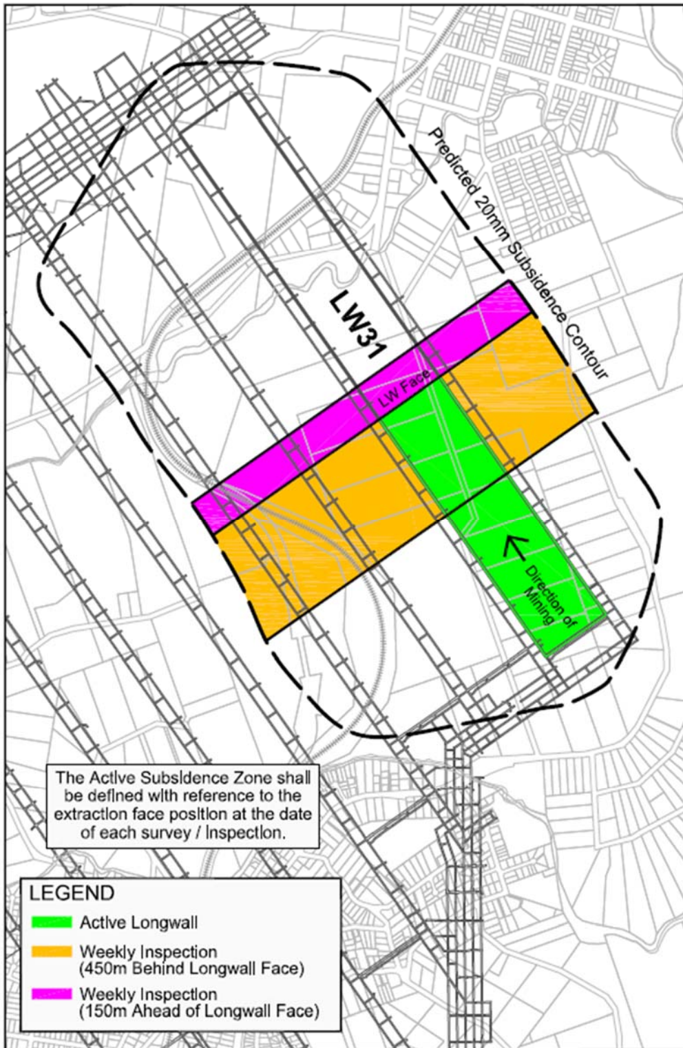
Fig. 1.1 Diagrammatic representation of the active subsidence zone
