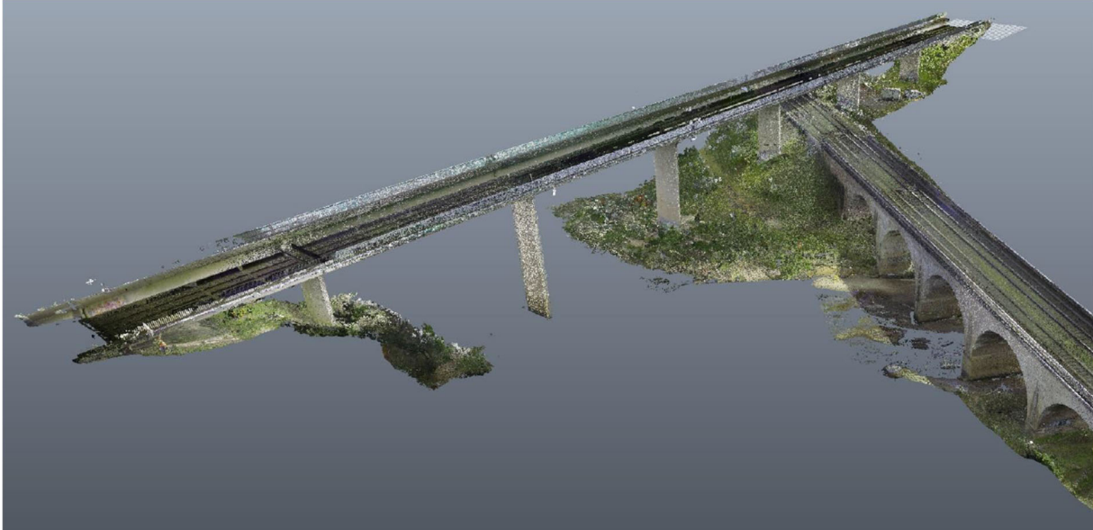
Fig. 3.29 Image produced from laser scan (Precision Surveys, 2022)
