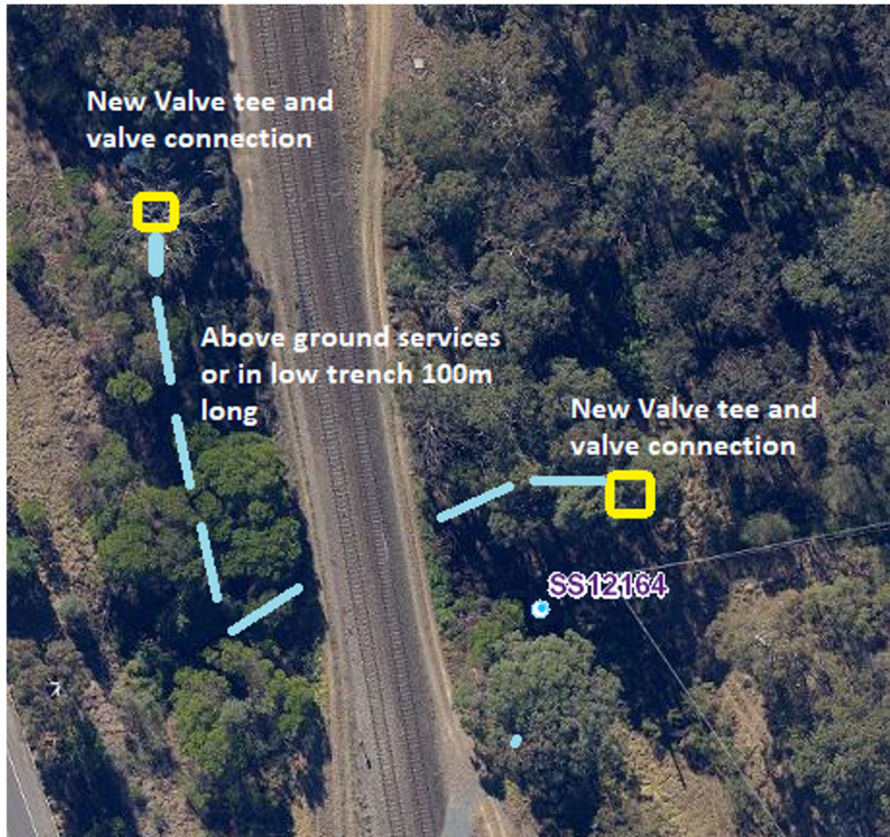
Fig. 3.15 Conceptual plan showing valve tees and connections to allow for emergency installation of a temporary bypass line
