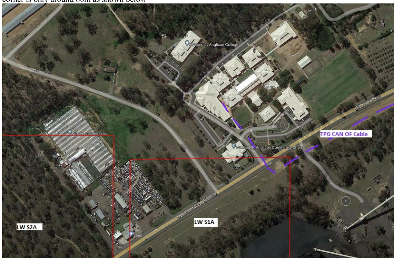
Plate 4: TPG CAN optical fibre cable from northern break-out joint along eastern side of Remembrance Drive and just crossing into the north-east corner of LW S1A before crossing Remembrance Drive to enter the Anglican College. The exposure length is approx. 80m.
