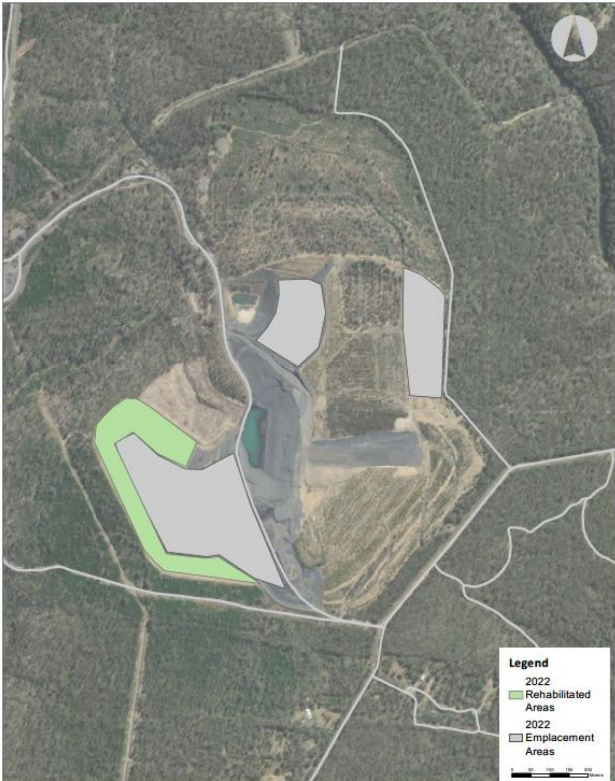
Figure 52 Reject Emplacement Areas and completed Rehabilitation works during 2022.
