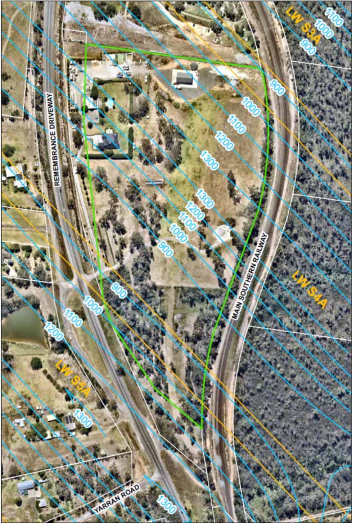
Fig. 3.1 Predicted Total Conventional Subsidence Contours after the extraction of LW S6A at No. 3165 Remembrance Drive, Bargo
