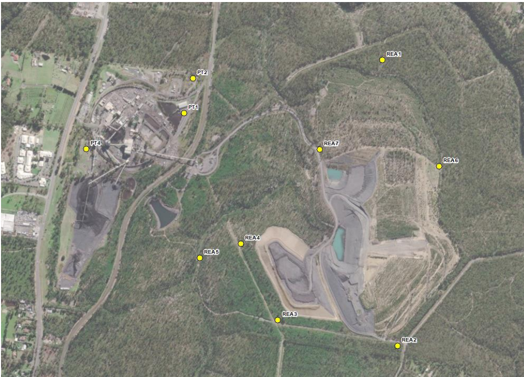
Figure 31 Locations of Piezometers at Pit-top and the REA areas
