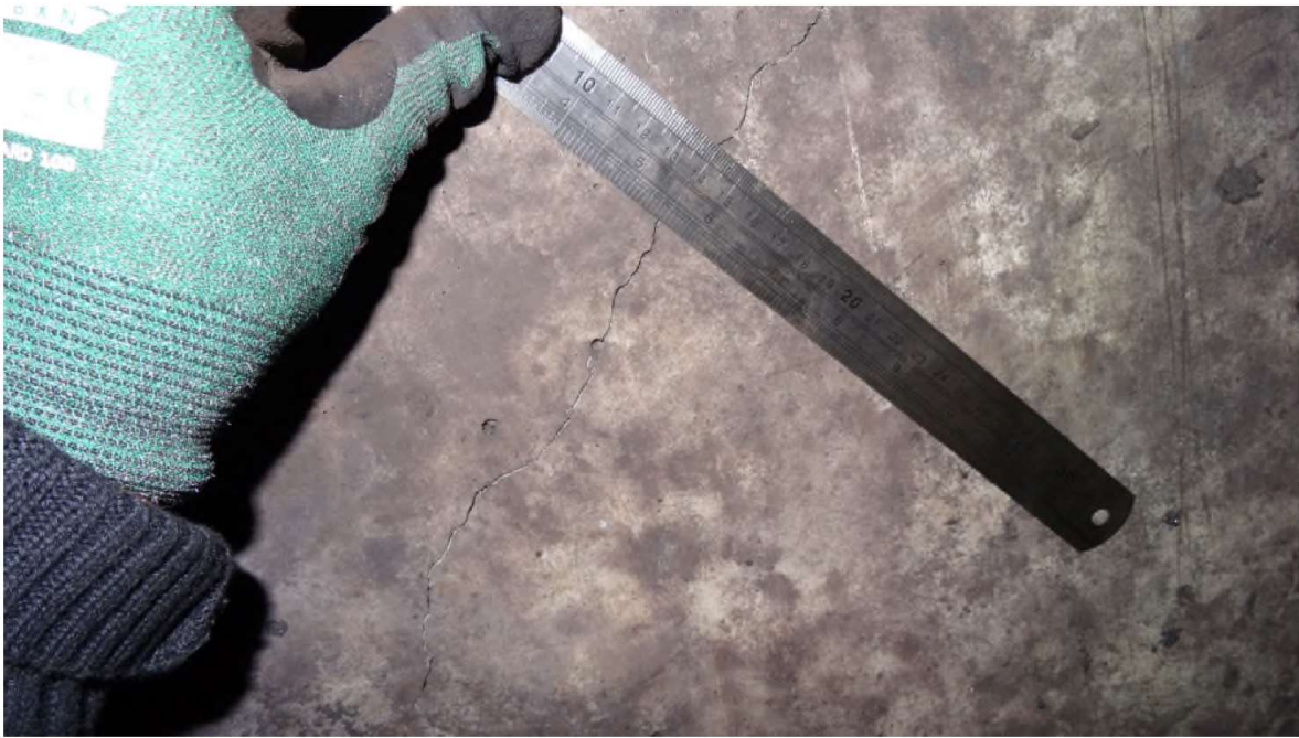
Plate 4.2 Crack B (C2), width <math><1\text{ mm}</math> (David Talbert 29 May 2023).
