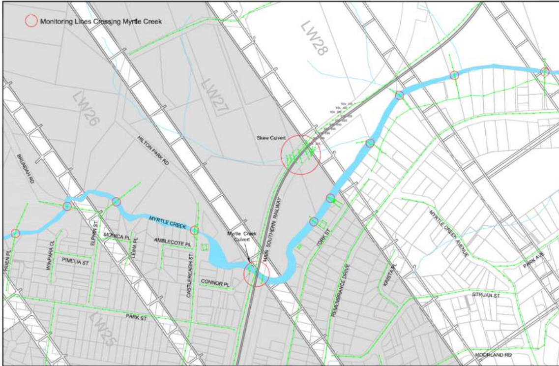
Fig. 3.10 Monitoring lines across Myrtle Creek and the Skew Culvert
