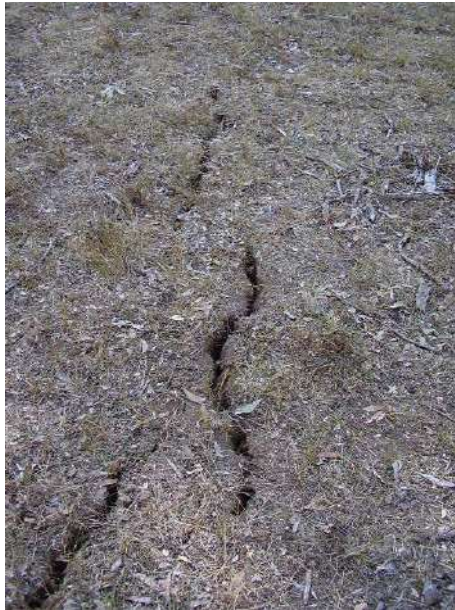
Fig. 4.11 Surface tension cracking along the top of a steep slope
