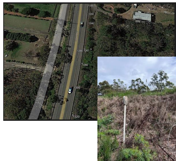
Figure 3-2: Plan view showing the sharp bends north of Teatree Hollow. Aerial photo showing Potholes #1267 and #1268 at the bends. Photo (below right) showing the buried pipe change in direction in the road embankment
