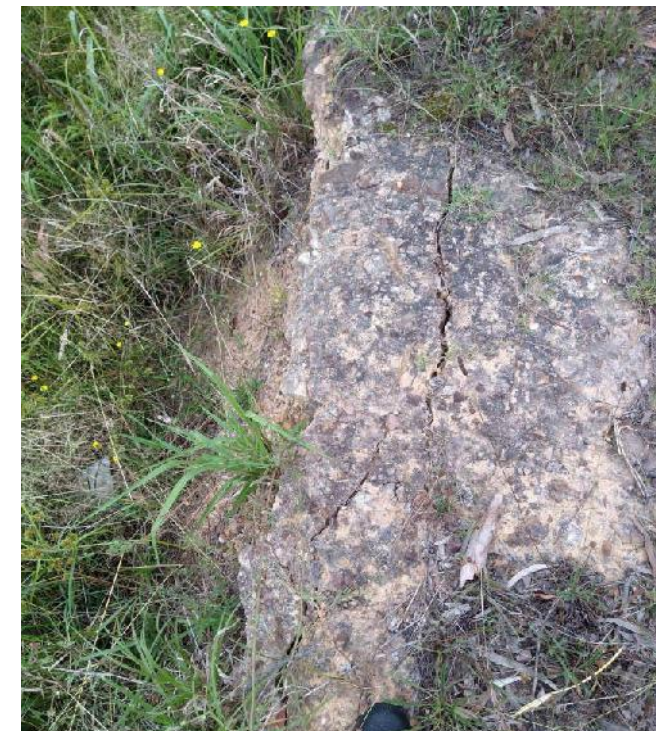
Photo 16: View looking at tension cracks setback behind the crest of opposite No. 3122 Remembrance Drive.
