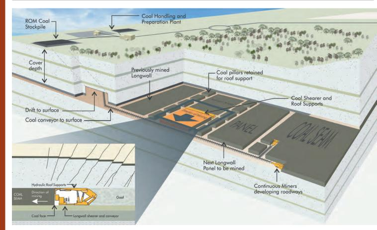
Figure 1: Schematic diagram of longwall mining
